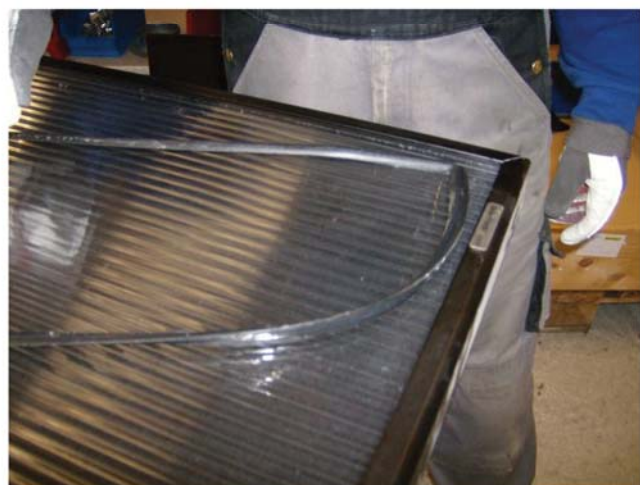
22. The rubber strip is put back in between the cover layer and the aluminum frame on the front. Begin from a corner.
