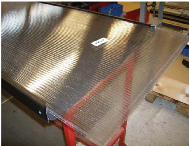
18. The cover layer is inserted, remember to put the front up.
