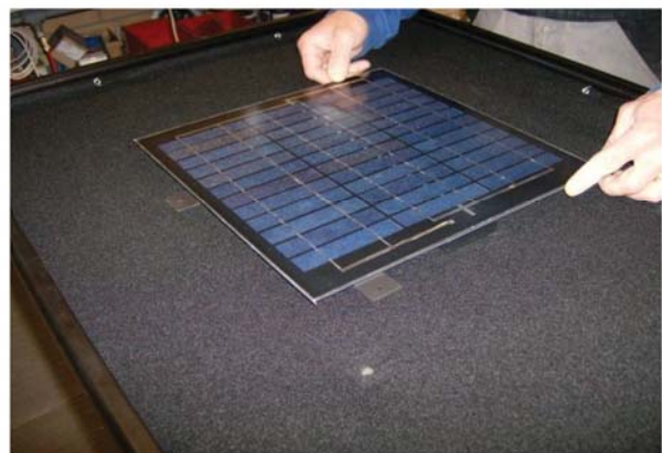
15. The solar cell is put in place.
