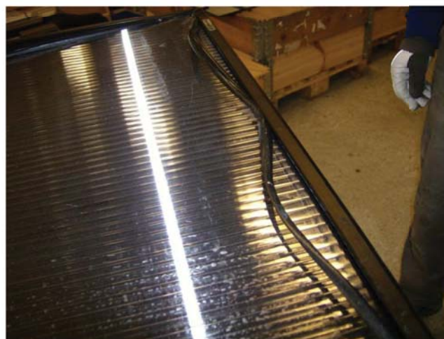
23. The rubber strip is then put in around the panel. Be aware that the rubber strip is "too long". This makes it possible to adjust itself when it's hot, cold etc.
