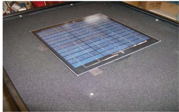
11. The "old" solar cell is replaced with the new blue solar cell.
